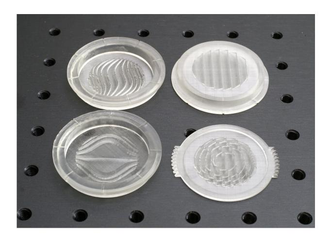
The two meta-devices on top are for 2D manipulation, the one on the bottom left is for testing, and the one on bottom right is a metasurface from a triplet metadevice. Credit: City University of Hong Kong
