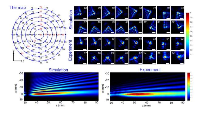
Comparison between a theoretical simulation and an experimental demonstration of the meta-device for varifocal THz beam generation, showing the high performance of the meta-device. Credit: City University of Hong Kong
