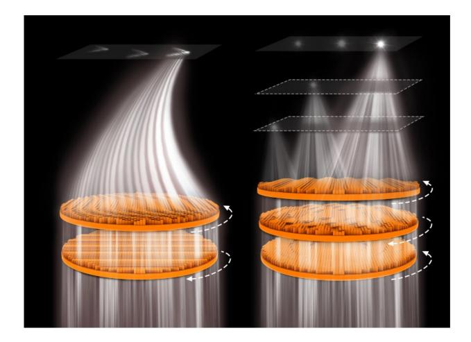
Schematic of the varifocal meta-devices: doublet (left) and triplet (right) metadevices. Credit: *Science Advances* (2023). DOI: 10.1126/sciadv.adf8478
