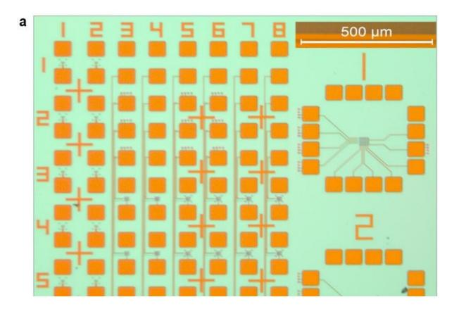
Devices and circuits in the microchip. a, Optical microscope image of the part of the microchip measured in this study, including standalone memristors (columns 1-2), standalone transistors (columns 3-8) and 5×5 crossbar arrays of 1T1M cells (right part), as-received from the foundry. b-c, Zoom-in optical microscope images of standalone h-BN memristor and standalone transistor before (up) and after (down) fabrication. Credit: *Nature* (2023). DOI:
