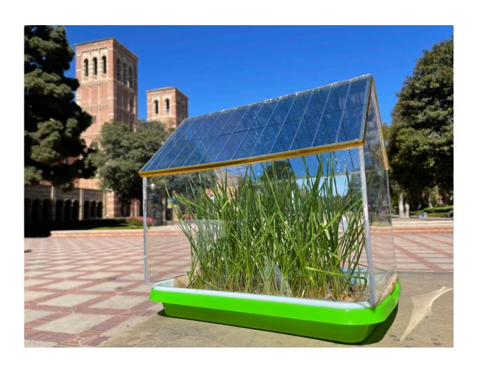
A miniature greenhouse prototype with its roof built of semi-transparent solar cells invented by UCLA materials scientists that resulted in better plant growth than a traditional greenhouse. Credit: Yang Yang Laboratory/UCLA
