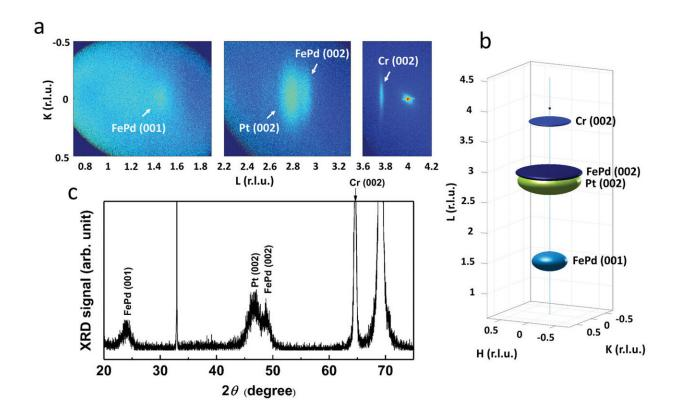
XRD patterns of the sample. a) Large area reciprocal space maps (HL projection). The scattered intensity is represented with a temperature-colored scale. b) The 3D representation of the 00L specular rod. In this representation, the scattering ellipsoids are obtained from the fitting of individual peaks in both the HL and KL projections. c) The conventional  $\theta$ –2 $\theta$  spectrum. Credit: *Advanced Functional Materials* (2023). DOI: 10.1002/adfm.202214201
