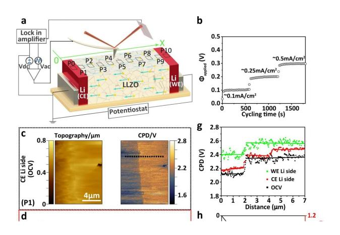
Operando KPFM measurements on LLZO close to electrode. **a** Schematic of KPFM on the LLZO surface of a symmetric LilLLZOlLi cell. The cell was cycled via a potentiostat. **b** Cycling performance of the symmetric LilLLZOlLi cell with potentials of 100, 200, and 300 mV applied to the Li-WE at the set constant current densities of 0.1 mA/cm<sup>2</sup>, 0.25 mA/cm<sup>2</sup>, and 0.5 mA/cm<sup>2</sup>. **c**-**f** Topography images and the corresponding CPD maps of OCV state, lithium
