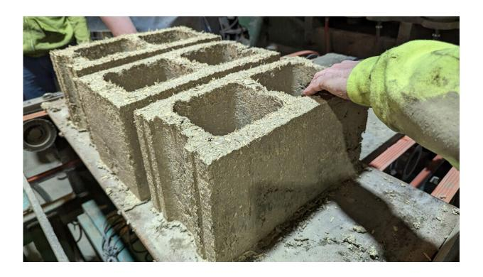
A Nebraska Engineering team has developed a hemp-based mixture for concrete masonry blocks that is lighter than traditional Portland cement but also meets the American Society for Testing and Materials' standards for strength, water absorption and weight. Credit: University of Nebraska-Lincoln
