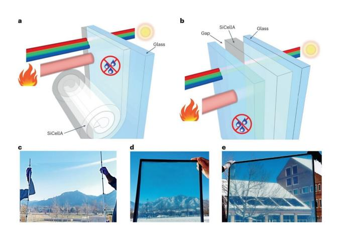
SiCellA-based window retrofits and IGUs. **a**,**b**, Schematic drawings of a window retrofitted with a SiCellA film (**a**) and an IGU with a SiCellA film inserted between glass panes (**b**). Schematics depict how window products can be used to boost thermal insulation and condensation resistance while maintaining visible-range transparency. **c**, Square-meter, 1.5 mm-thick SiCellA with 99.2% porosity adhered to an optically clear plastic film. **d**,**e**, Photos of 36 cm × 51 cm (**d**) and
