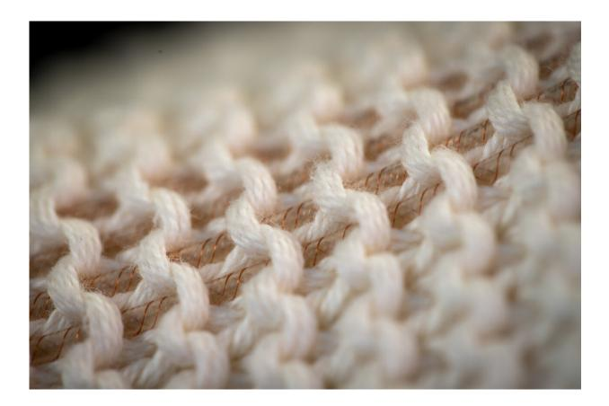
The fiber pumps knit into fabric. Credit: LMTS EPFL
