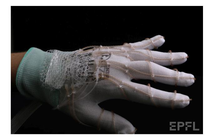
A thermal haptic glove, created with fiber pumps. Individual fiber pumps are sewn to each finger of the glove, each connected to a reservoir of chilled fluid on the back of the hand. Each fiber pump can be activated separately, causing
