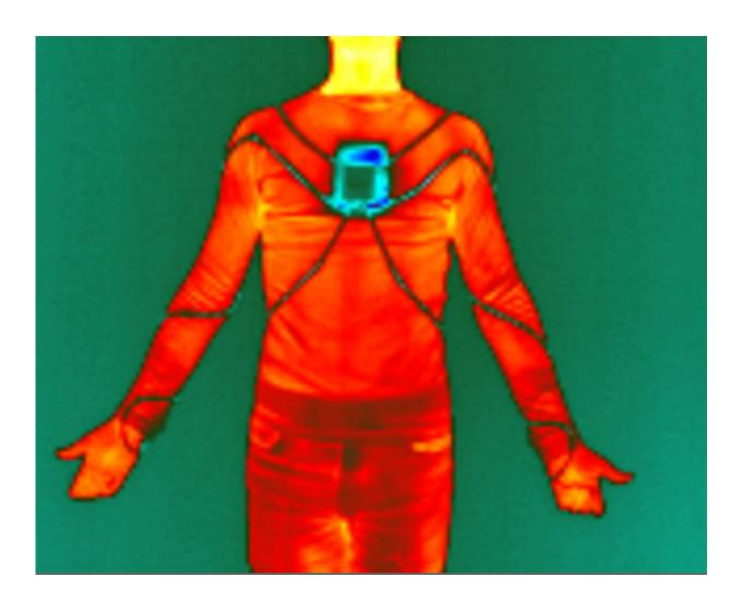
Infrared image of the pumps integrated into a t-shirt. Credit: © LMTS EPFL
