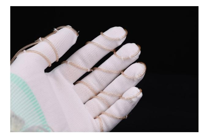
The pumps integrated into a glove. Credit: © LMTS EPFL
