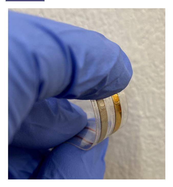
This flexible, miniature pH sensor can be put on food packaging using existing methods, such as plastic wrapping, to detect food wastage. Credit: SMU
