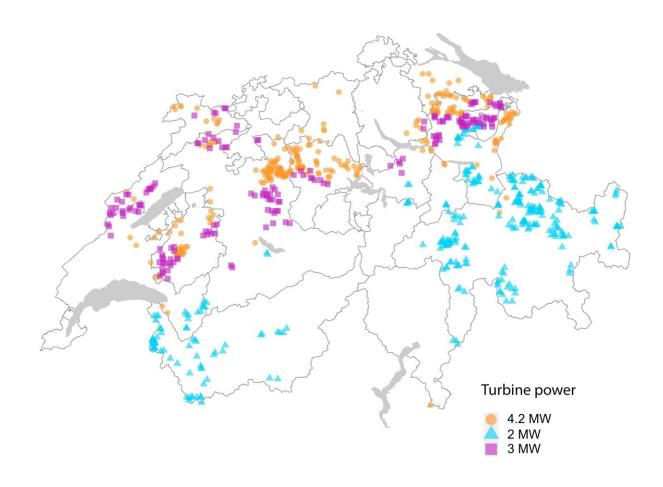
Optimal distribution of wind power sites based on the current wind energy concept. Orange circles: largest wind turbines on the Swiss Plateau. Purple squares: medium-sized turbines in the foothills of the Alps and in the Jura Mountains. Turquoise triangles: smaller turbines in the Alps. Credit: Reto Spielhofer / ETH Zurich
