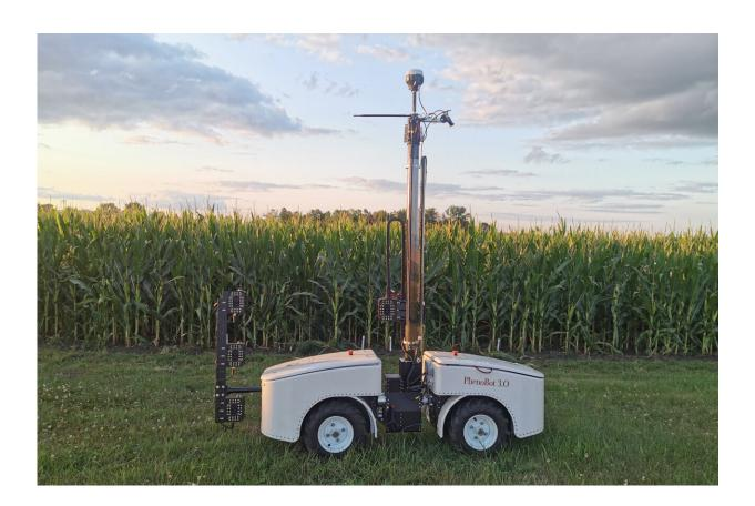
This image shows the autonomous robot, with multiple tiers of PhenoStereo cameras, that are part of the AngleNet system. Credit: Lirong Xiang, NC State University
