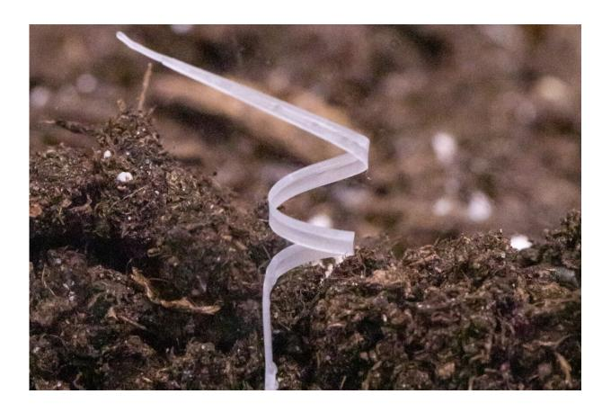
The first I-Seed created at IIT is inspired by the seed structure of a South African geranium, the Pelargonium appendiculatum, whose ability to change shape in reaction to variations in humidity in the surrounding environment, the so-called hygromorphic structure, is replicated. Credit: IIT-Istituto Italiano di Tecnologia
