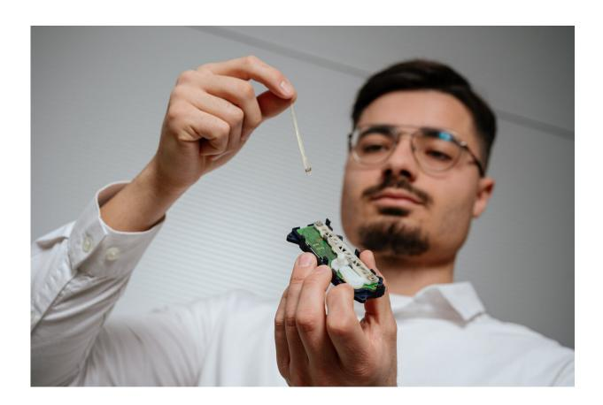
Researchers are using artificial muscles made from nickel-titanium alloy to build compact technical components. Doctoral student Carmelo Pirritano is currently researching these novel smart drive systems. Credit: Oliver Dietze
