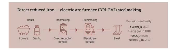
This figure shows what's involved in making green steel using the direct reduced iron-electric arc furnace process. Credit: Australian Industry Energy Transitions Initiative, Author provided
