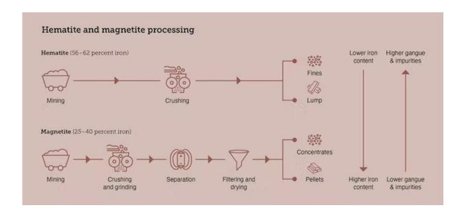
This chart shows a comparison between hematite and magnetite processing. Magnetite processing requires more steps but produces a product more compatible with current green steel methods. Credit: Australian Industry Energy Transitions Initiative, Author provided
