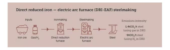
This figure shows what's involved in making green steel using the direct reduced iron-electric arc furnace process. Credit: Australian Industry Energy Transitions Initiative, Author provided
