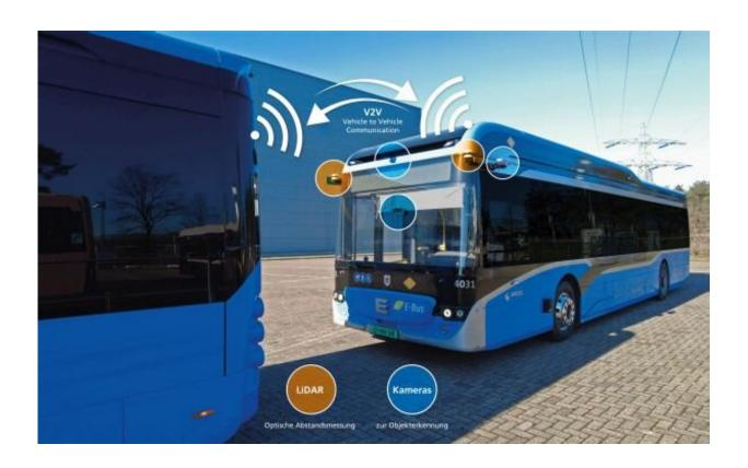
Electronically networked traffic: With platooning, bus convoys can be connected or split up as needed. Credit: ITIV, KIT
