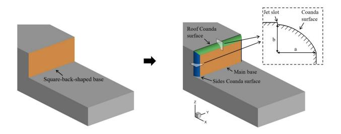
One of the main sources of aerodynamic drag is the square-shaped back of the ship's superstructure. The Chalmers researchers have created a superstructure design with convex edges and highly compressed air flowing through "jet slots". The Coanda effect then allows the air pressure on the ship's hull to be balanced out which, in turn, considerably reduces aerodynamic drag. Credit: Chalmers University of Technology | Kewei Xu
