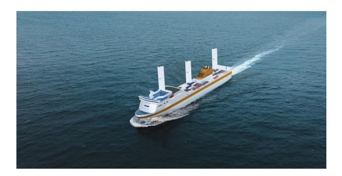
Illustration of a wind-powered ship. Its wing sails are one of the designs that can be used to harness wind power for large ships. Other design types include rotor sails (which look like vertical cylinders) and kite sails. Credit: computedwingsail.com
