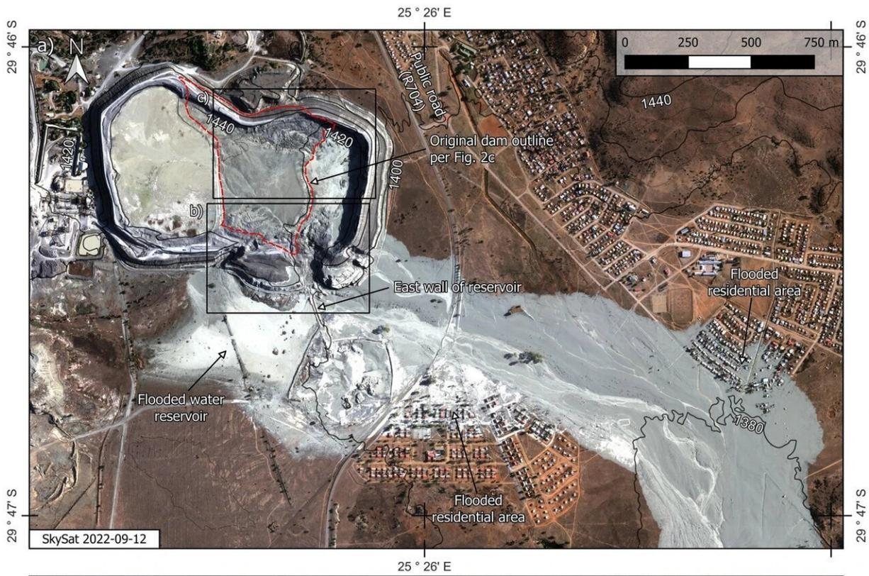
The post-failure scenario. (a) Impact on the immediate surroundings. (b) Enlargement of breached area. (c) Enlargement of collapsed northern wall. (d) Full extent of the tailings runout. Credit: *Scientific Reports* (2023). DOI: 10.1038/s41598-023-31633-5
