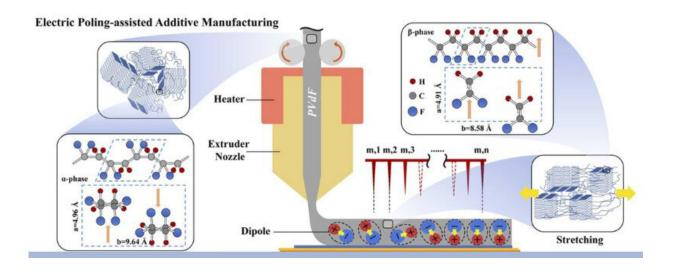
Purdue University researchers have combined 3D printing and electric poling into a single process called electric poling-assisted additive manufacturing, or EPAM. It aligns the dipoles in PVdf filament during the printing, which leads to a better indication of the stress being applied. Credit: Purdue University/Robert Nawrocki
