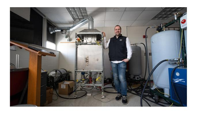
Prototype of the flameless impingement oven built by Pawel Olszewski in the engineering and engineering technology department at UW Oshkosh. Olszewski recently was granted a U.S. patent for the oven, which mixes air and flammable gas in such a way that it creates heat without visible flame. Credit: UW Oshkosh
