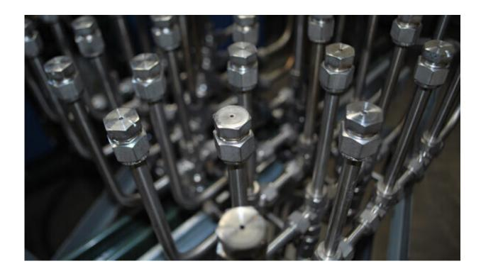
The flameless impingement oven prototype features 25 air nozzles and 16 natural gas nozzles. Once ignited, the oven produces temperatures beyond 1,000 degrees Celsius. Credit: University of Wisconsin Oshkosh
