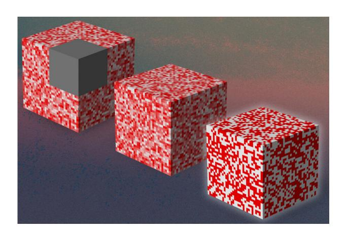
A machine-learning method developed at MIT detects internal structures, voids, and cracks inside a material, based on data about the material's surface. On the top left cube, the missing fields are represented as a gray box. Researchers then leverage an AI model to fill in the blank (center). Then, the geometries of composite microstructures are identified based on the complete field maps using another AI model (bottom right). Credit: Jose-Luis Olivares/MIT and the researchers
