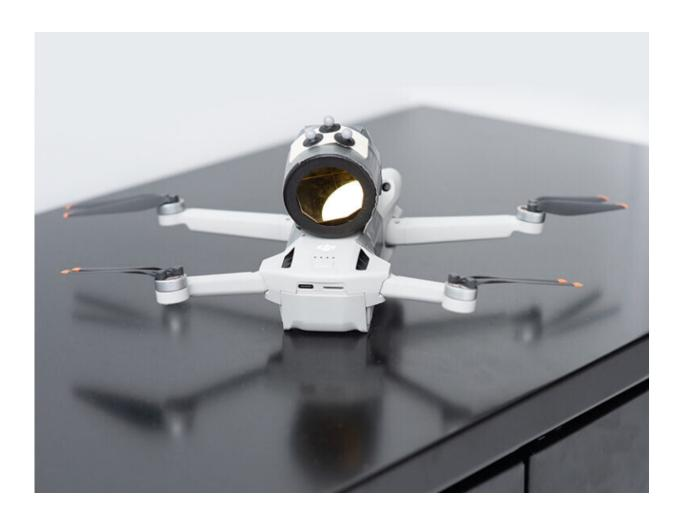
The retroflector mounted onto the drone. Credit: Bumper DeJesus, Princeton University
