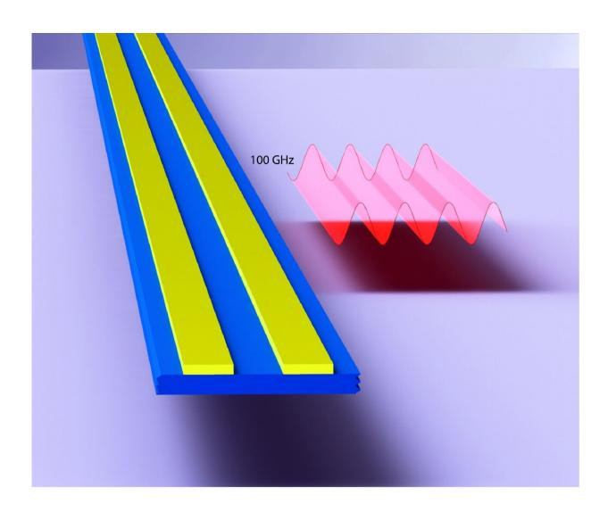
Suspended lithium niobate mechanical resonator vibrating at 100 GHz. Credit: Xie et al
