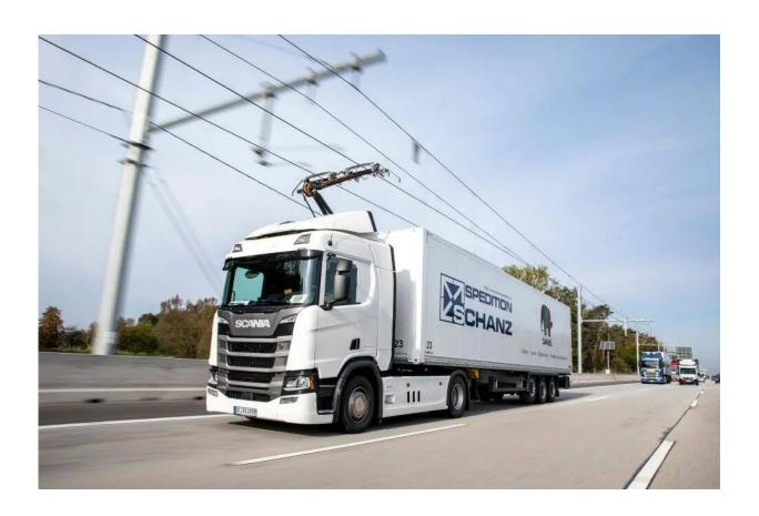
Siemens Mobility built an overhead contact line for electric trucks on a 6.2-mile stretch of Germany's autobahn. Credit: Siemens
