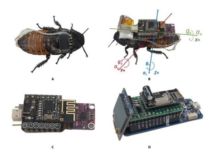
Scientists from Osaka University designed a cyborg cockroach and optimized its movement by utilizing machine learning-based automatic stimulation. Credit: *Cyborg and Bionic Systems*
