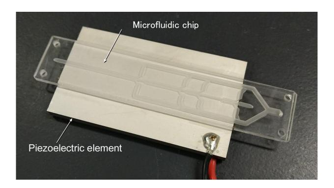
The device developed by researchers from Japan has four serial trifurcated junctions where a 500 kHz acoustic wave is applied for a 105-fold enrichment of various-sized microplastics in water. Credit: Yoshitake Akiyama from Shinshu University
