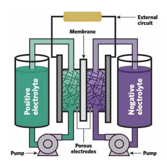
In a flow battery, negative and positive electrolytes are pumped through separate loops to porous electrodes separated by a membrane. During discharge, electrons
