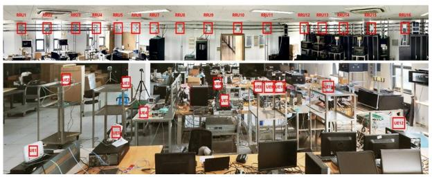
On the top, schematic diagram of the prototype full-spectrum CF-RAN system; On the bottom,test scenario of a low-frequency CF-RAN. Credit: Science China Press
