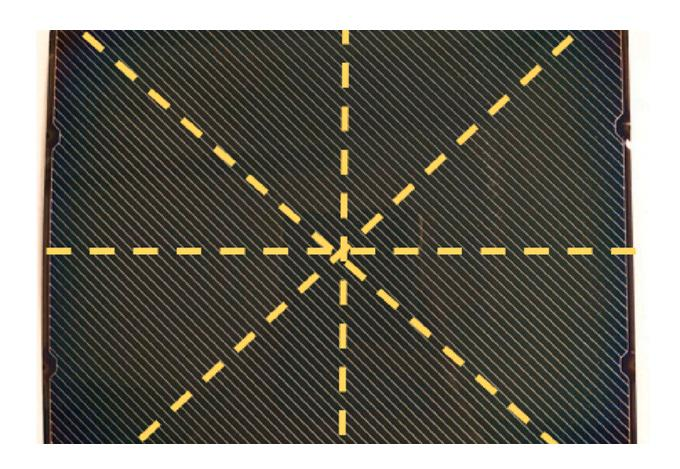
a) Division of a flexible CIGS solar cell  $(15.6 \times 15.6 \text{ cm}^2)$  into 8 identical samples and b) the way of cutting further each sample used in the experiments. Credit: *Solar Energy Materials and Solar Cells* (2023). DOI: 10.1016/j.solmat.2022.112178
