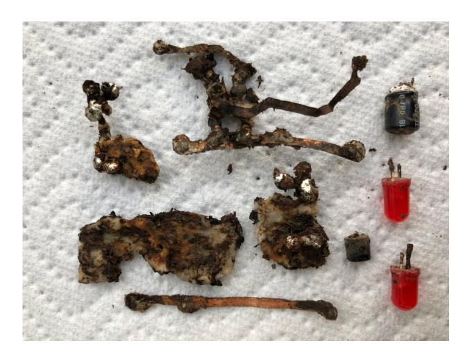
Biowaste: Experimental board after composting. Credit: Empa
