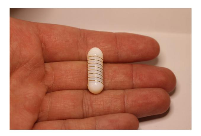
An ingestible capsule that delivers an electrical current can stimulate the release of the hormone ghrelin. Developed at MIT, the capsule could prove useful for treating diseases that involve nausea or loss of appetite, such as anorexia or cachexia. Credit: Khalil B. Ramadi et al
