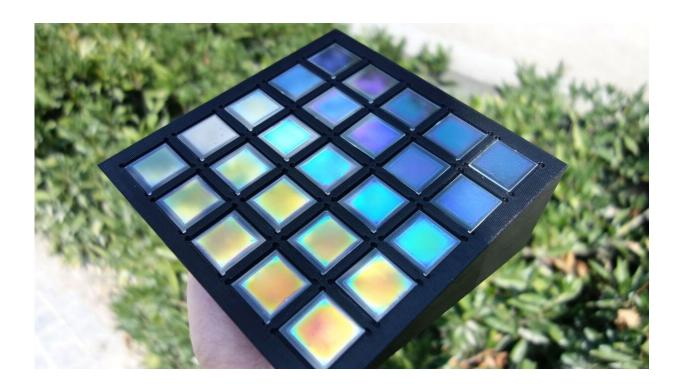
Inkjet-printed optical filters can be used to control optical properties precisely. Credit: LTI, KIT
