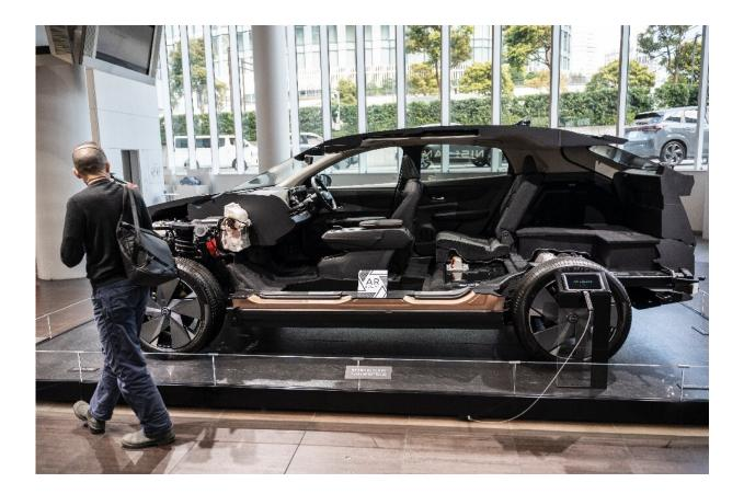
A cutaway display model of one of Nissan's electric vehicles seen at the global headquarters of Japanese automaker Nissan Motor in Yokohama.
