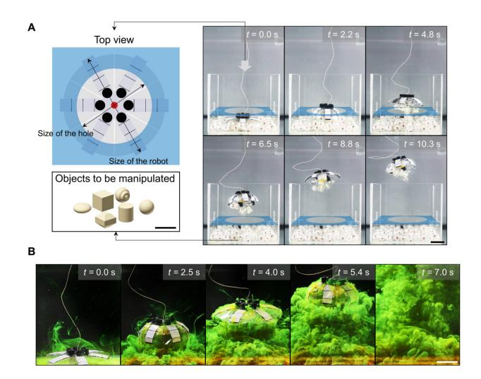
Contactless manipulation of irregular-shaped objects and dye. (A) Shape adaptation of the robot to transport objects of various shapes out of a confined space (f = 1 Hz, D = 0.7; movie S2). The space was composed of a box and a plate on the top with a central hole. The diameter of the hole (13 cm) was smaller than the outer diameter of the robot (16 cm). (B) Visualized fluidic
