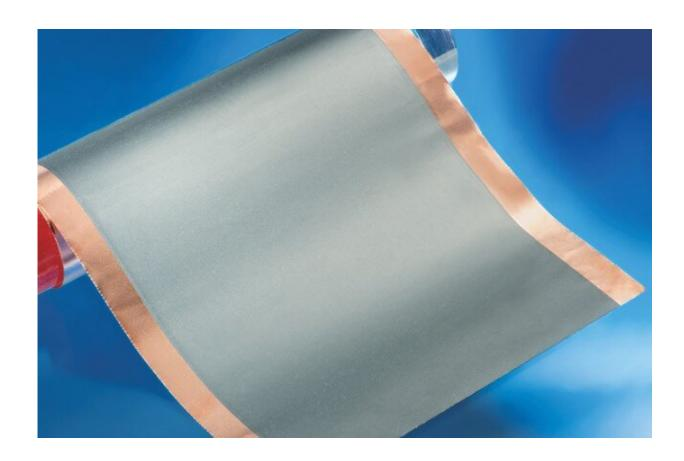
Electrode layer applied to copper foil and dried with laser technology: Researchers at Fraunhofer ILT have halved the energy required for drying in the production of lithium-ion batteries. Credit: Fraunhofer ILT
