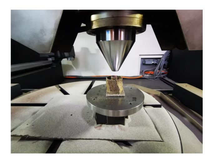
Direct energy deposition machine adapted by Skoltech researchers for printing metal foam. Credit: Oleg Dubinin/Skoltech
