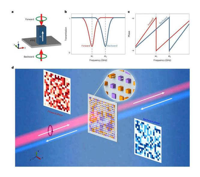
a) Operation mechanism of a self-biased magnetic meta-atom. b) Non-reciprocal transmission near Mie resonance modes, leading to non-reciprocity in the
