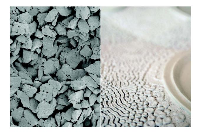
Probiotic ceramic tiles embedded with a soil derived microbe that can inhibit harmful bacteria. Left: Microscale image of porous ceramic material. Right: Geometrical surface details of probiotic pores with porous and non-porous zones. Credit: Richard Beckett
