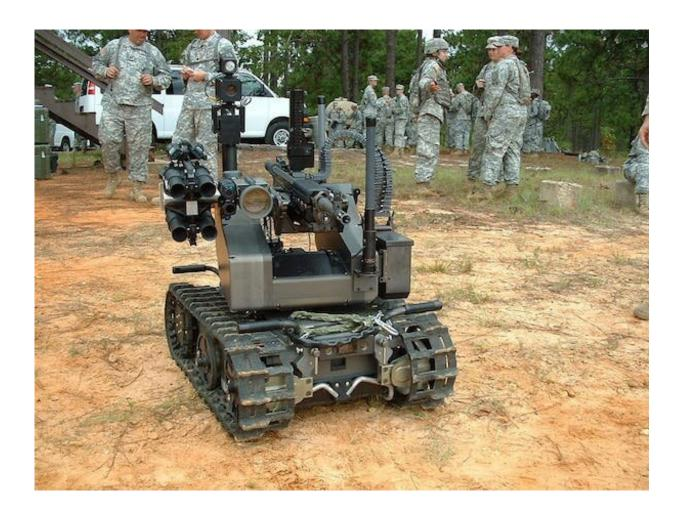
This US military robot is fitted with a machine gun to turn it into a remote weapons platform. Credit: US Army
