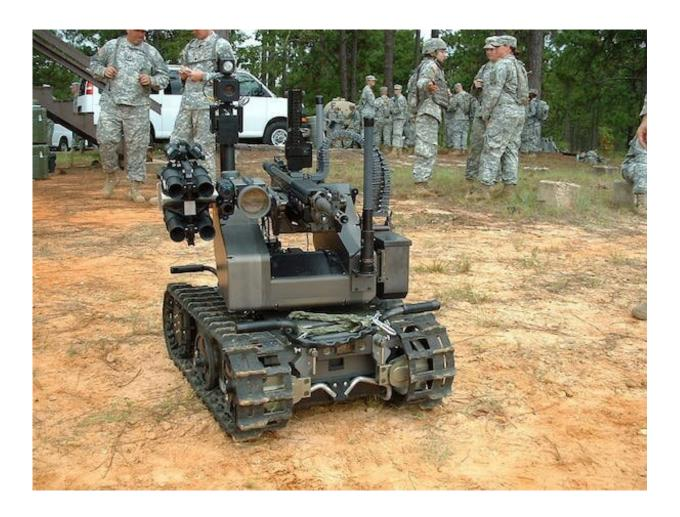
This US military robot is fitted with a machine gun to turn it into a remote weapons platform. Credit: US Army
