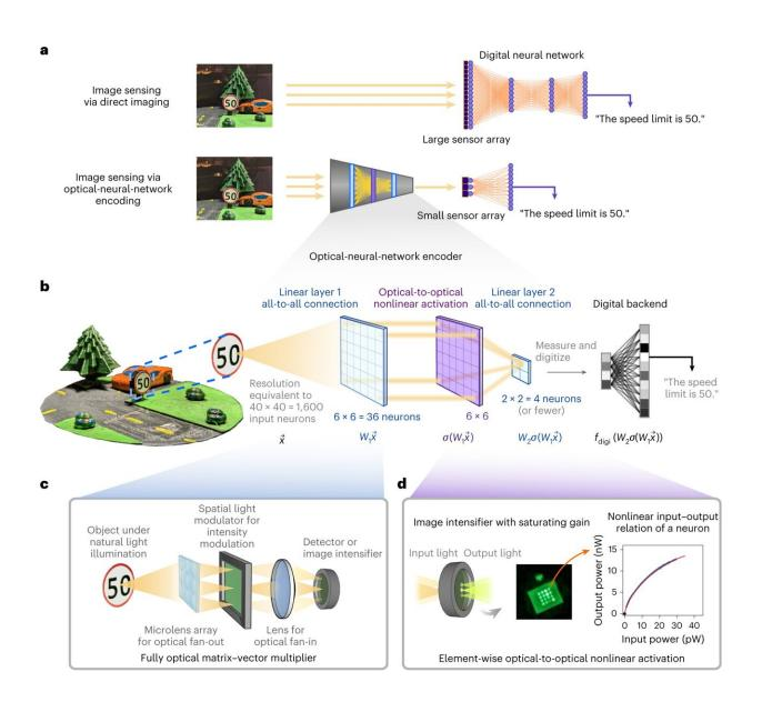
A multilayer optical-neural-network encoder as a frontend for image sensing. Credit: *Nature Photonics* (2023). DOI: 10.1038/s41566-023-01170-8
