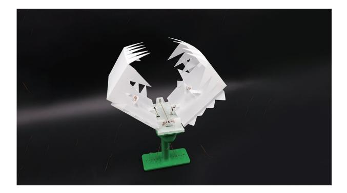
A Venus flytrap-like robot that envelops a "prey" when both of its jaw sensors detect an object. Credit: UCLA Samueli
