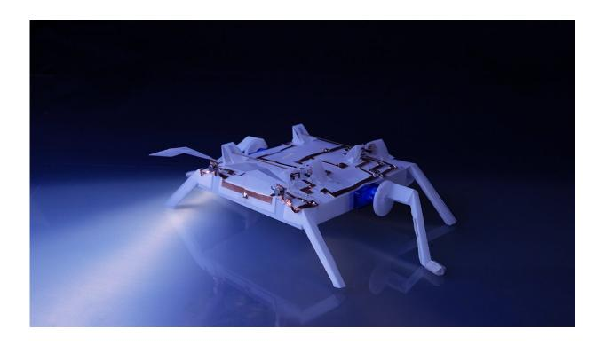
An origami-inspired robot designed by a UCLA-led team that can reverse direction when either of its antennae senses an obstacle. Credit: Wenzhong Yan/UCLA
