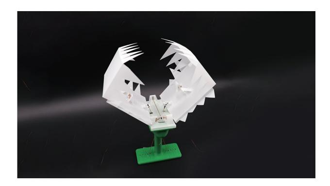
A Venus flytrap-like robot that envelops a "prey" when both of its jaw sensors detect an object. Credit: UCLA Samueli
