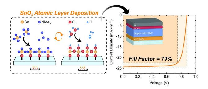
This image shows the production of the new organic solar cells using Atomic Layer Deposition. The tin is deposited using a precursor chemical (NMe<sub>2</sub>) and oxygen is added through  $H_2O$ , while the temperature is used to tune the optical and structural characteristics of the tin oxide layer. Credit: Loi Lab, University of Groningen
