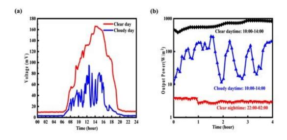
(a) The self-powered TEG can produce electricity on clear and cloudy days. (b) The normalized electric power generated by the device under three different conditions. Credit: Haoyuan Cai, Jimei University
