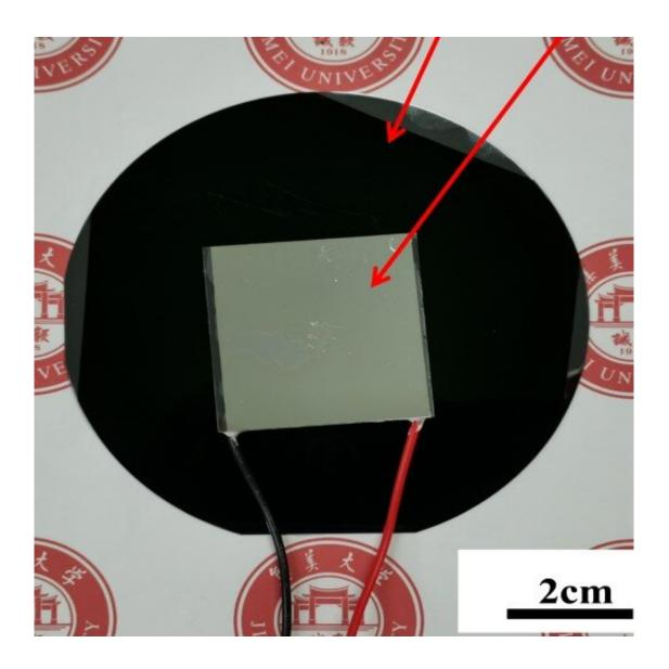
The new self-powered thermoelectric generator device uses an ultra-broadband solar absorber (UBSA) to capture sunlight, which heats the generator. Simultaneously, another component called a planar radiative cooling emitter
