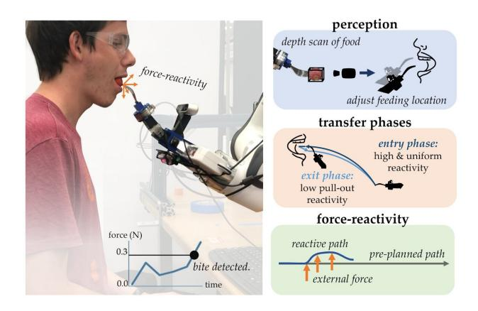
Algorithms combine haptics and computer vision to evaluate how to insert a fork into a person's mouth naturally and comfortably. Credit: Stanford University
