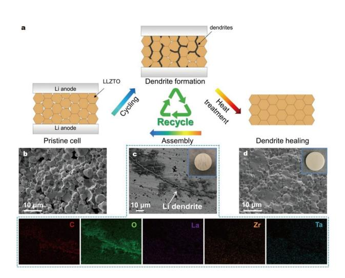
(a) Schematic diagram showing the formation and healing process for Li dendrites. (b) Cross-sectional SEM image of the pristine LLZTO pellet. (c) Cross-sectional SEM image and the corresponding EDS mapping of the LLZTO pellet with dendrites (inset: optical picture of the LLZTO pellet with dendrites).
