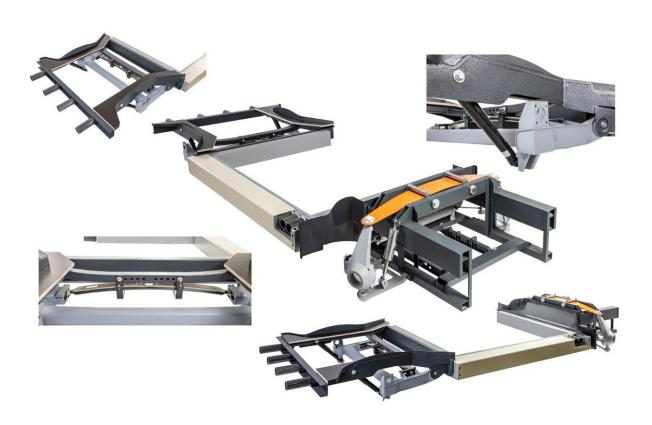
The sill consisting of crash absorbers in the form of carbon fiber-reinforced plastic (CFRP) tubes and a buffer element with an auxetic polyurethane structure provides protection both for the passengers and for the energy source, namely the battery or hydrogen tank. Credit: Fraunhofer-Gesellschaft
