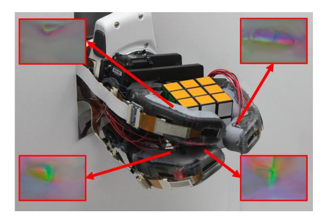
MIT researchers developed a soft-rigid robotic finger that incorporates powerful sensors along its entire length, enabling them to produce a robotic hand that could accurately identify objects after only one grasp. Credit: Massachusetts Institute of Technology
