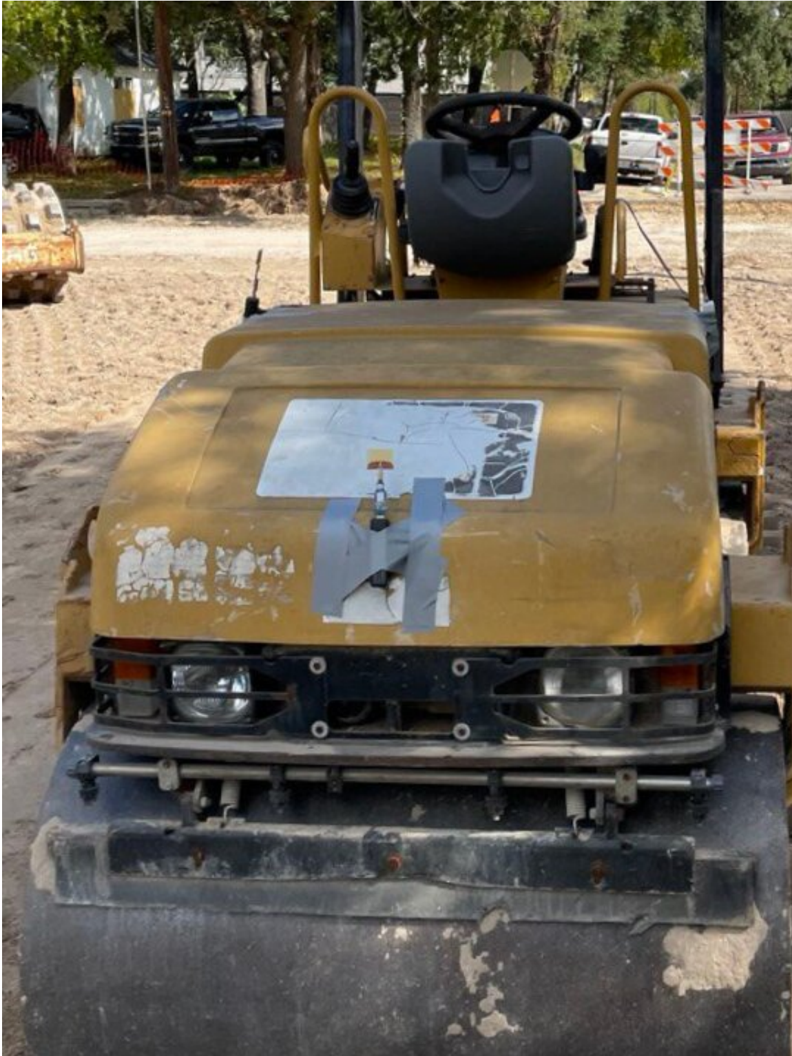
Construction truck with a ultra-wideband tag that allows students to monitor its location. Credit: University of Houston
