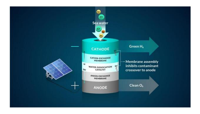
A representation of the team's bipolar membrane system that converts seawater into hydrogen gas. Credit: Nina Fujikawa / SLAC National Accelerator Laboratory
