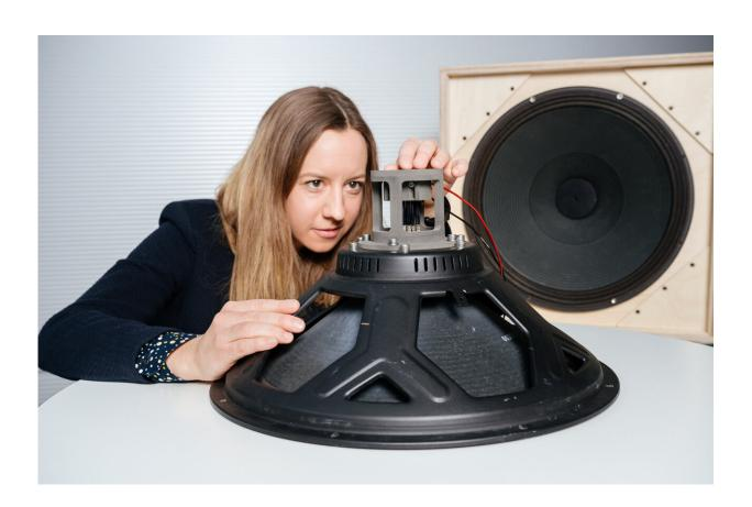
Smart films can now be used as a new type of speaker driver, replacing the electromagnets or permanent magnets that drive the loudspeaker membranes in conventional speaker systems. But the film can also be made to generate acoustic tones—essentially turning it into its own loudspeaker. Sophie Nalbach conducted research into these smart polymer films as part of her doctoral thesis in Professor Stefan Seelecke's group. Credit: Oliver Dietze
