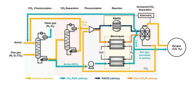
Schematic diagram comparing the novel CO2 utilization technology(the proposed reaction swing absorption(RSA) pathway) with conventional CCU pathways. Credit: Korea Institute of Science and Technology
